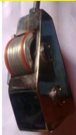
The FDC-35-F uses flat type rubber stereotypes for printing.
